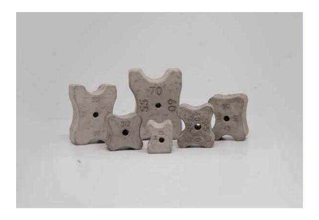
Multi Cover Concrete Spacers are manufactured from glass fibre reinforced cement, and are as strong as the surrounding concrete. They are recommended for use in vertical applications and the design allows excellent concrete flow and minimise the area of spacer at the surface. They are strong, durable, and the optimum choice for heavy-duty steel fixing applications.
