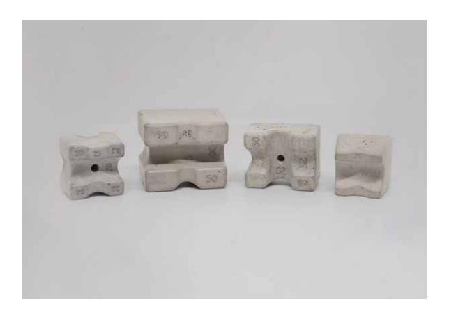
Concrete Flat Base Spacers are manufactured from glass fibre reinforced cement, and are heavy-duty concrete spacers Ideal for supporting reinforcement on polyethylene membranes ,blinding and horizontal form work.
