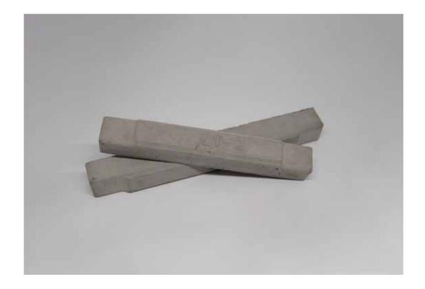
Concrete Square Bars are manufactured from glass fibre reinforced cement, in different lengths with a variety of square sections. Fixing costs are greatly reduced as the bars can simply be laid on the form work or ground floor sub-base prior to the loading of the reinforcement cage.
